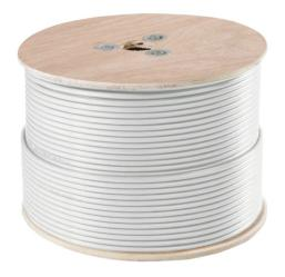
Use the video combination cable to connect individual components and ensure high-quality data transmission. The two integrated power wires (2x 0.75mm<sup>2</sup>) supply connected equipment with electricity. The cable impedance is 75 0hm. The video combination cable is available in three lengths: 50 m (KA9002), 100 m (KA9001) and 250 m (KA9000).
