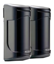
This innovative Profiline infrared light beam detects up to a distance of 60 m indoors and 30 m outdoors. Dual light beams and anti-sabotage monitoring of the transmitter and receiver guarantee reliable functionality. A special plus: Installation is quick and easy thanks to the horizontal and vertical alignment capabilities of the transmitter and receiver, laser beam calibration, and LED display.
