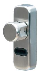
This reliable and robust cylinder provides secure, controlled and convenient access. It was specifically designed for use with panic doors with automatic reset of the locking nose. It is operated using the read-protected ABUS Seccor chip key. The reader is double-sided, meaning that identification is required in both directions when opening the door.
