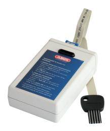
The transfer device is a bidirectional interface between tags and the administration PC. On the one side tags are read into the PC or recorded events are transmitted. Locking and arming rights are transmitted to the locking systems in the other direction.
