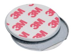
The magnet fastening set offers an ideal alternative for smoke alarm device installation - without the need for screws and wall plugs. The set consists of a self-adhesive plate for mounting on the ceiling and a base element for mounting on the smoke alarm device, with the two magnetic parts holding the detector securely in place. This means that quick, easy and tidy installation is possible, without having to drill holes or use additional tools.
