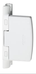
The ABUS FAS97 additional lock is intended for securing the hinge side of a window. You should secure the opening side separately. Locking is automatic so there is no need to activate the additional lock manually. When you open the window, the FAS97 moves with it; to tilt the window, simply push the hinged bar to the side. The hinge side lock is mounted on the casement and on the frame. Because it locks automatically when the window is closed, the lock is always engaged.
