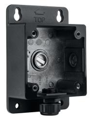
The Installation Box is an optional accessory for the IP Mini Dome IPCB42510A/B/C, IPCB42515A, IPCB44510A/B/C. If the Wall Mount TVAC31450X is fitted together with the Installation Box, the latter will house the connecting cables, providing protection and insulation for the cabling against moisture both indoors and out. This provides the best possible level of protection for the cable, ensuring it is not affected by environmental factors or tampering.
