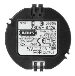
The stabilised mini clip built-in power supply unit (230 V AC / 5 V DC, 2 A) is used to supply power to your video components. The enhanced version with a lever spring clamp means that quick installation is possible without the need for a tool or an additional clamp. Its compact dimensions mean that it is especially suitable for use as a flush mounted power supply for installation in a 55 mm flush socket and anywhere there is limited space available for the power supply.
