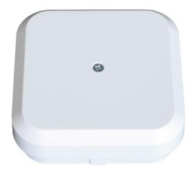
This wireless receiver unit receives its commands directly from the CLX, SLT or ZL door systems wirelessly. It passes these commands on to the evaluation unit AE255F via a wire connection which is connected to the alarm system in turn. This makes wireless incorporation of the door systems possible without additional door wiring.
