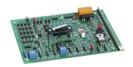
Intelligent circuits for more security and comfort are realised with the AE255F evaluation unit. It is thus possible to specify in a targeted way which people may arm, disarm or use both functions. Users who only have access in a disarmed state can also be created. It is also possible to apply special codes for silent alarms, internal arming or special keys for the guard users.
