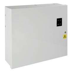
The CCTV performance power supply transforms 230 VAC into 13.8 VDC. It is therefore ideal to serve as central power supply station for video surveillance systems. The device provides 8 separate connections.
