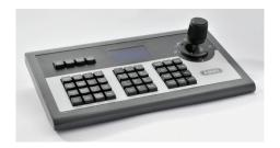
Help yourself! Controllable video surveillance for analogue cameras. This ergonomically designed and robustly made control panel enables simple control of up to 255 motor domes via RS-485. The integrated LCD display enables you to monitor each of your control steps. One special feature is the additional option to directly control several recorders. Direct access to the OSD of the connected dome is also possible. With the ABUS DVR control panel you can manage up to 31 recorders simultaneously.
