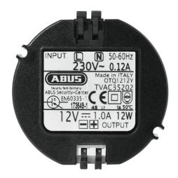
The stabilised mini clip built-in power supply unit (230 V AC / 12 V DC, 1 A) is used to supply power to your video components. The enhanced version with a lever spring clamp means that quick installation is possible without the need for a tool or an additional clamp. Its compact dimensions mean that it is especially suitable for use as a flush mounted power supply for installation in a 55 mm flush socket and anywhere there is limited space available for the power supply.
